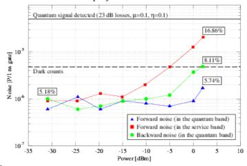
Figure 2. Forward and backward noise measurements.
