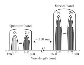
use of not only one channel per port, but also its periodic "harmonics". Therefore, we slice the quantum and service bands in subbands that match the periods of the AWG, such that each QKD pair can use such periodically matching channels from both bands to communicate. The scheme is easily implemented using standard commercial components. A test bed network of three access networks and a span of 16 km has been deployed in order to test this scheme.
