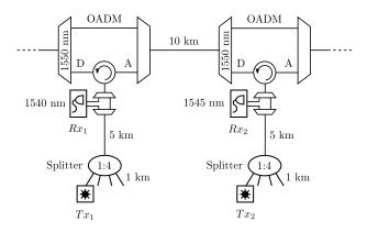
Fig. 12. Alternative scheme of a QKD-PON with circulators instead of bandpass filters. This reduces the number of components, but signals can travel only in the forward direction. This means that, to recover the connectivity with the previous node, accessible in the scheme of Fig. 10, either the quantum signal has to travel the full ring in the forward direction till reaching the node before or a second ring running in parallel but in the backward direction must be used.
