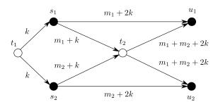
Fig. 5. This figure shows a network with two sources  $s_1$  and  $s_2$ and two users  $u_1$  and  $u_2$ . The sources,  $s_1$  and  $s_2$ , transmit  $m_1$  and  $m_2$  to the users,  $u_2$  and  $u_1$ , respectively, while no information is leaked to the intermediate nodes or the remaining users.
