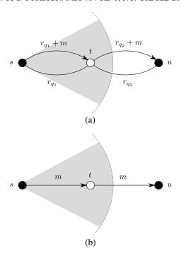
Fig. 7. The reach can be extended by allowing trusted intermediate nodes to forward the key. The gray area marks the distance limitation of the QKD system with the emitter source at s. (a) Detail of the messages exchanged with a trusted repeater. (b) Logical schema of a link extended with a trusted repeater.
