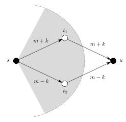
Fig. 8. The scenario corresponds to an optical network with two disjoint paths that are used to overcome the QKD distance limitation. As in Fig. 7, the gray sector marks the distance limitation of the QKD system with the emitter source at s.
